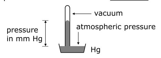
Pressure of atmosphere can support a 760 mm column of Hg
