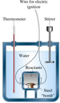
To measure the energy of combustion of  $C_8H_{18}$ , 0.5269 g  $C_8H_{18}$  are burned in a bomb calorimeter that has a heat capacity of 11.3 kJ/°C. If the calorimeter's temperature increases 2.25 °C, find  $q_{comb}$  in kJ/mol  $C_8H_{18}$
